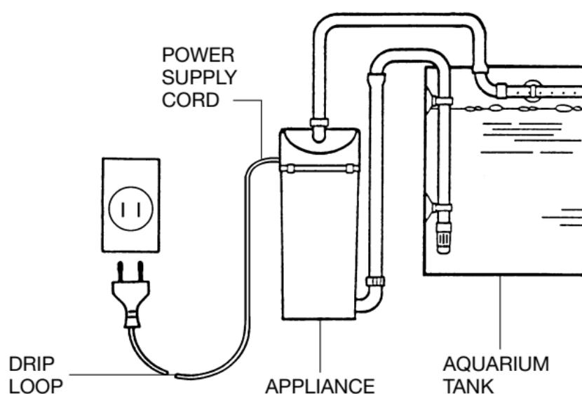
A "drip-loop", shown in the figure, should be arranged by the user for each cord connecting an aquarium appliance to a receptacle.
