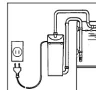
**When using a multiple socket or an external power supply unit, position them atop the filter's power connection.**
